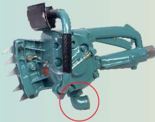
Underwater chain saw shown with exhaust valve.
